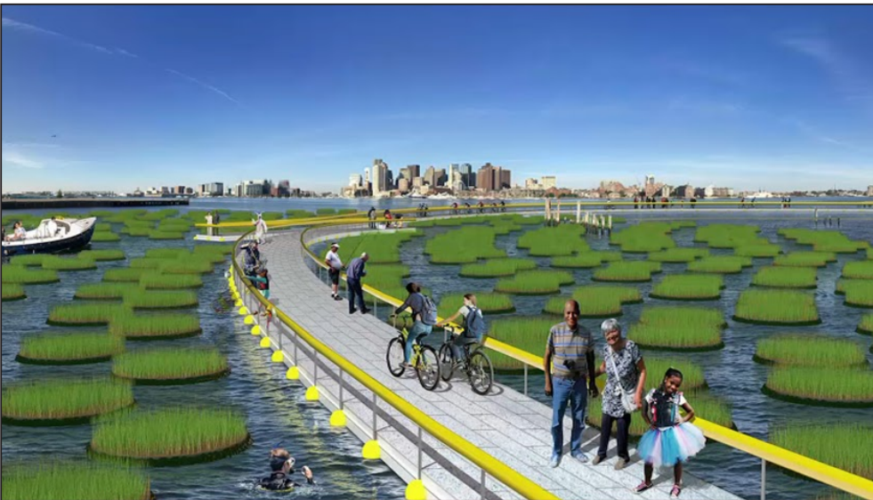
The goal is to have a floating network of interconnected, anchored massive organic growing modules that dampens wave energy and reduces flooding, storm damage, and erosion on shore while improving nearshore water quality.
